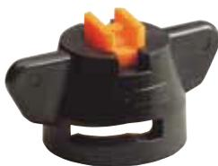
This nozzle has an 80° spray angle. On boom sizes from 80 ft to 132 ft the boom height is often higher than 20" above the target. 80° nozzles provide good coverage with reduced drift risk at these higher boom heights and are also adaptable to band spraying.
